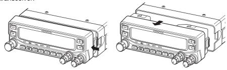
3 Flip the front panel upside-down, then reattach it to the main body of the transceiver.
